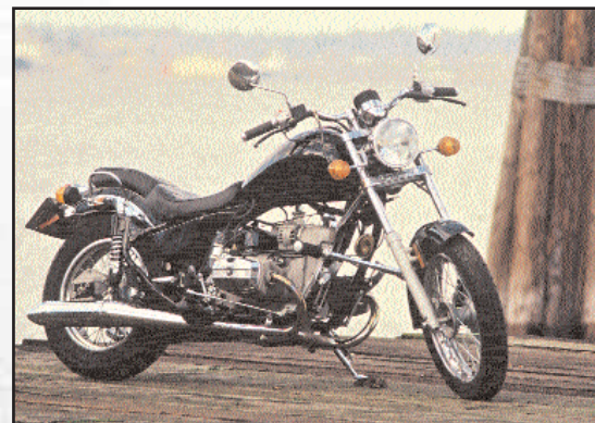
^ (top) Post-modern Ural features hydraulic Brembo disc and rear drum. (middle) Gear Up cargo area holds tire pump, Jerry can and a trenching tool. A transfer case powers sidecar wheel at the push of a lever. (bottom) 750cc Wolf honors the "Night Wolves" (Russia's version of the Hells Angels) motorcycle club with 18" front and 16" rear wheels, Paioli extended forks, and kick or electric start.
